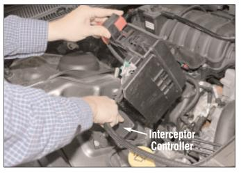
Place Interceptor Controller on its side in the compartment. Then re-install the fuse box back to its original location.
