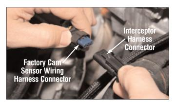
Plug the Interceptor harness connector into the factory cam sensor wiring harness connector.
