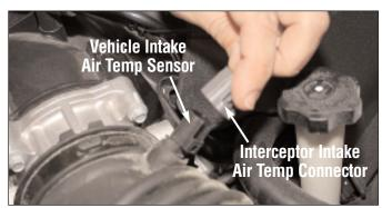
Plug the Interceptor intake air temp sensor connector into the vehicle intake air temp sensor.
