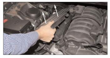
Lift off the passenger side engine cover.
