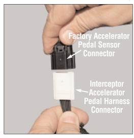
Plug the Interceptor accelerator pedal harness connector into the vehicle's factory accelerator pedal sensor connector.
