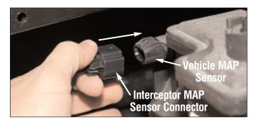
Plug the Interceptor MAP sensor connector into the vehicle MAP sensor.
